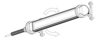
3) Tighten the screws using hexagon wrench.
